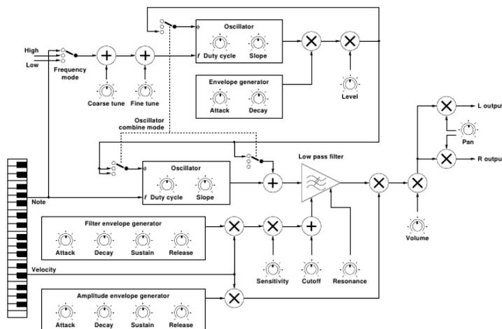
One point of interest is that each oscillator waveform is controlled by a pair of continuous parameters rather than, for example, a multi-position switch. The waveform is divided into four parts: a rising slope, a flat period, a falling slope, and a final flat period. Each slope takes the shape of half a cosine wave: the first
